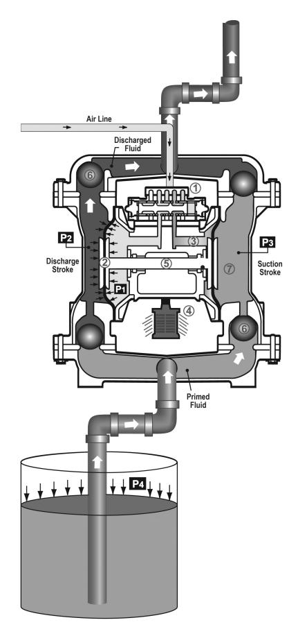
SANDPIPERP SANDPIPERPUMP.COM s30mdl1sm-rev1222 Air-Operated Double Diaphragm (AODD) pumps are powered by compressed air or nitrogen.
