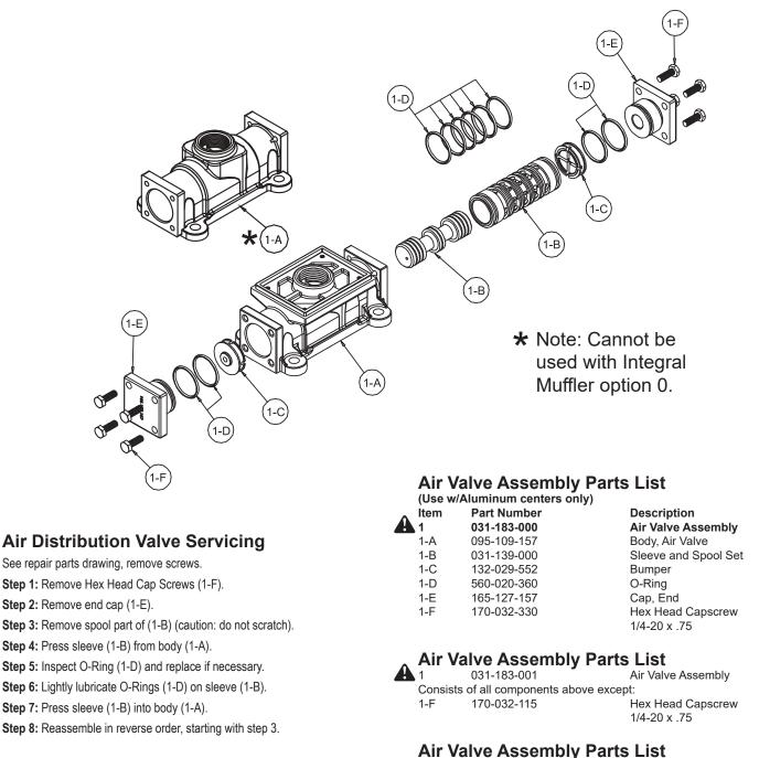
Note: Sleeve and spool (1-B) set is match ground to a specified clearance sleeve and spools (1-B) cannot be interchanged.
